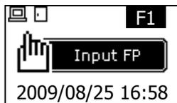
When you place the finger on the fingerprint sensor, the fingerprint input window is lighted in red along with "ppik" sound. Leave the finger until the light is switched off.
